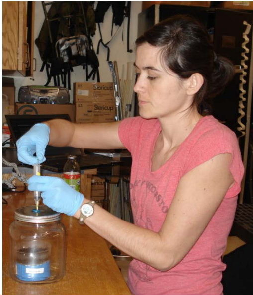
Sampling CO 2 during the lab incubation
