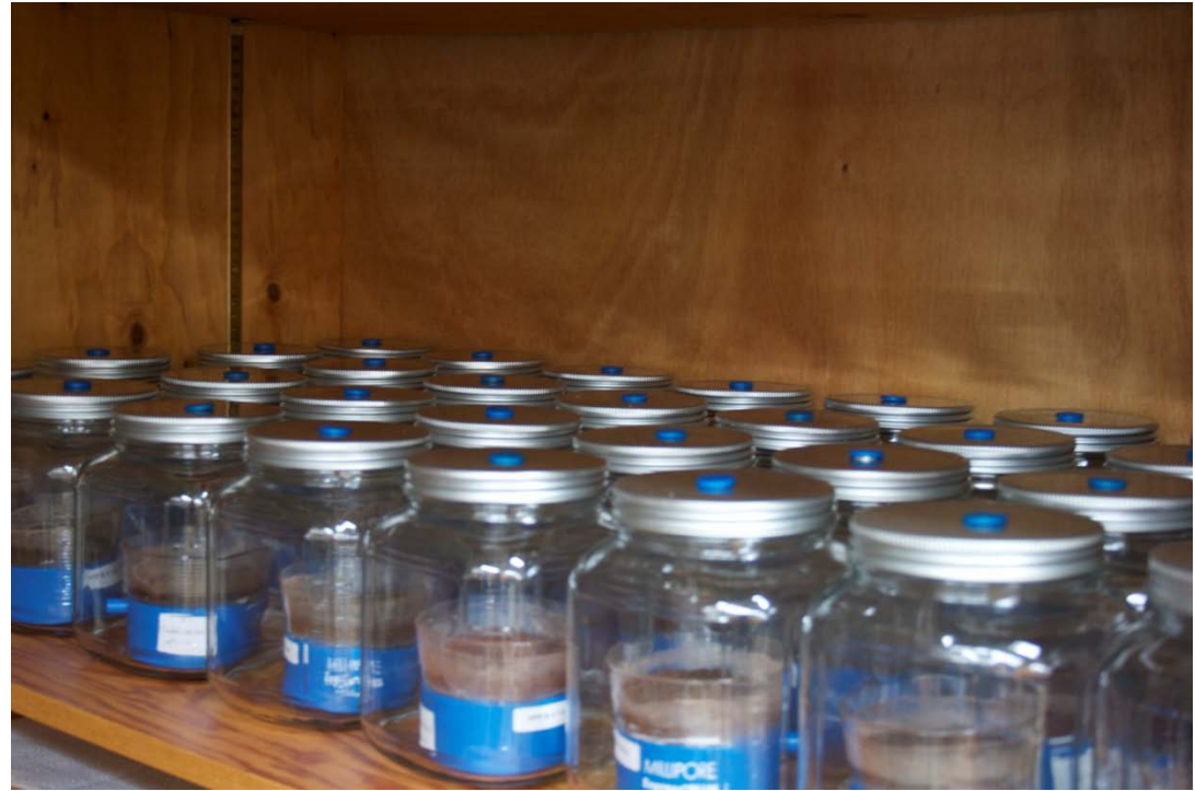
Soil samples sealed in jars for measuring release of carbon dioxide in the laboratory.
