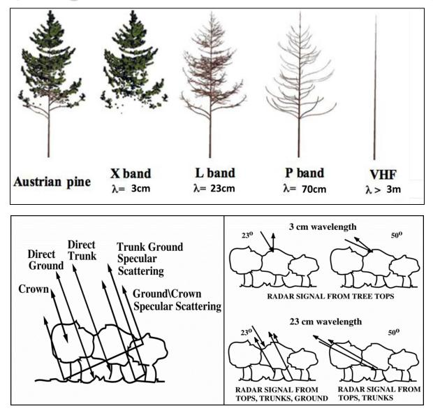
Illustrated is wavelength, penetration, and sensitivity to Austrian pine and scattering mechanisms and viewing geometry relationships.
