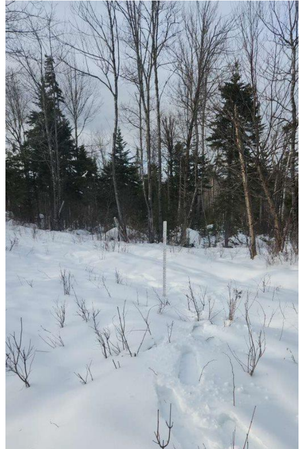
A camera site. There is a stake in the set up within the cameras view in order to measure snow depth. There is a turkey feather attached to the top to help attract wildlife to the camera.
