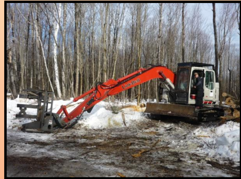
Machine operator getting ready to start up feller-buncher after fixing a broken hydraulic hose.
