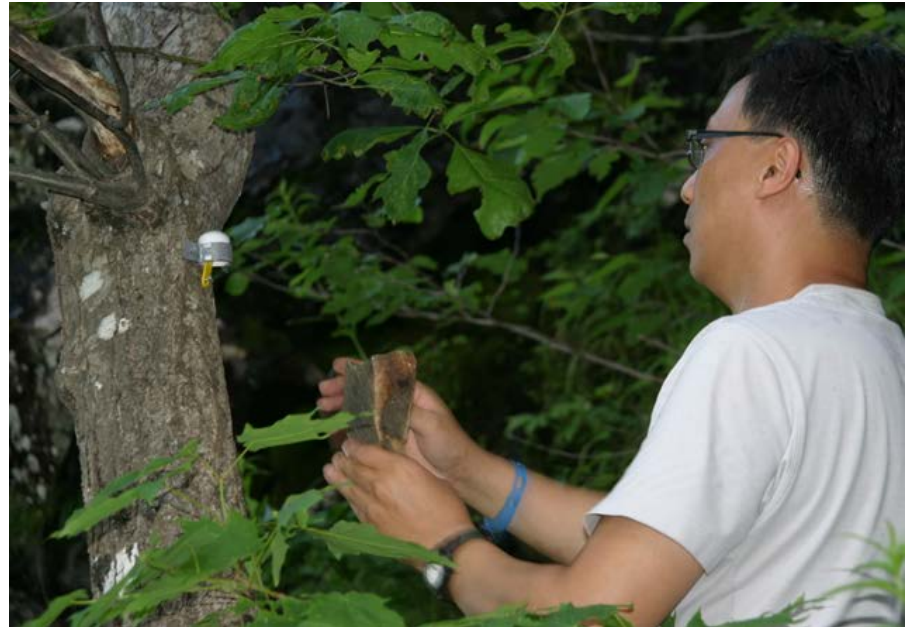
Figure 6. Installation of I-button temperature logger at site ME-SB.
