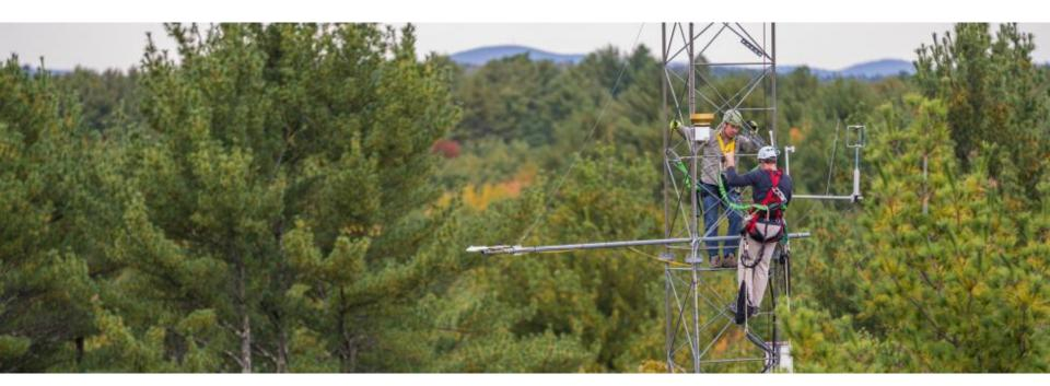
Eddy covariance flux towers with sensors located above the forest canopy measured the fluxes of carbon and water between forests and the atmosphere (top-down approach). These towers simultaneously recorded a suite of meteorological data which helped determine the climate drivers of ecosystem fluxes.
