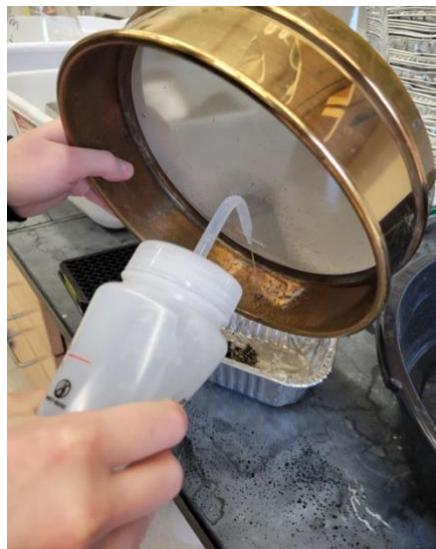
Figure 5. The particulate soil fraction (>53 microns) being rinsed off a sieve, separating the soil into particulate and mineral-associated fractions to understand how these different soil carbon pools are affected by timber harvesting in arbuscular and
