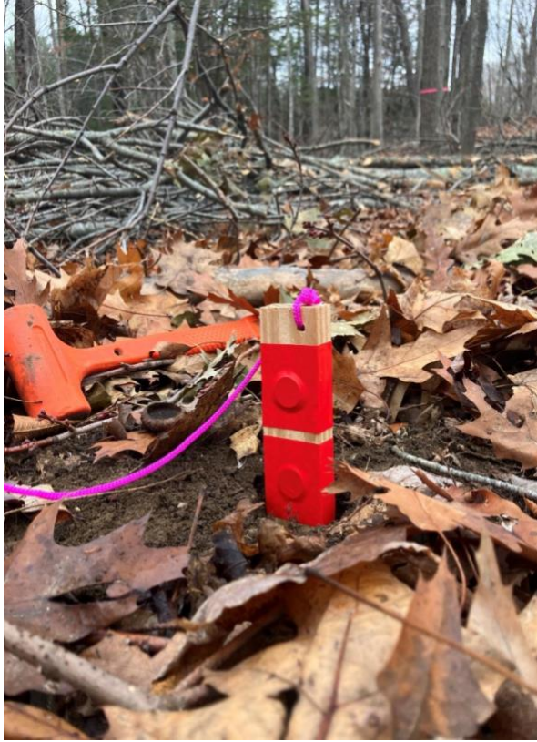
Figure 21. Soil sensors (iButtons) to be installed below grade under a corduroy crossing (photo by Shannon Van Hise)
