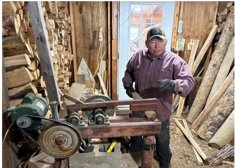
Figure 8. Basketmaker Richard Silliboy demonstrating his ash pounding machine for research team members.
